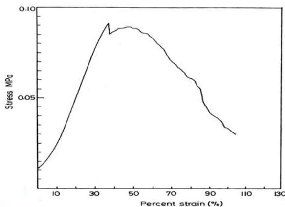
Fig. 3a: Stress-strain curve uncross linked collagen - Chitosan matrix
