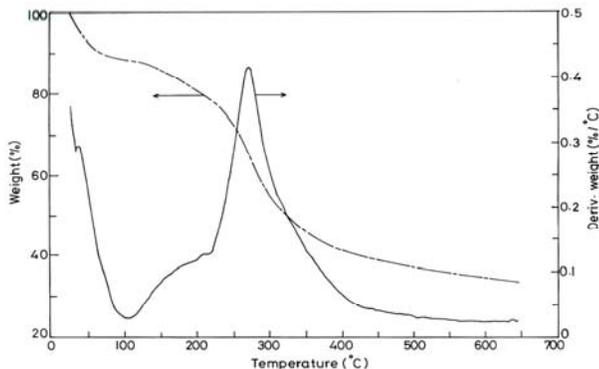
Fig 4a: Thermal decomposition pattern of uncross linked collagen - Chitosan matrix
