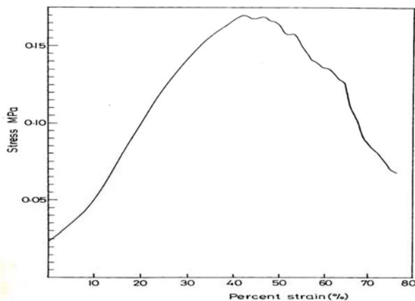
Fig. 3b: Stress-strain curve cross linked collagen - Chitosan matrix
