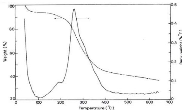
Fig. 4b: Thermal decomposition pattern of cross linked collagen - Chitosan matrix
