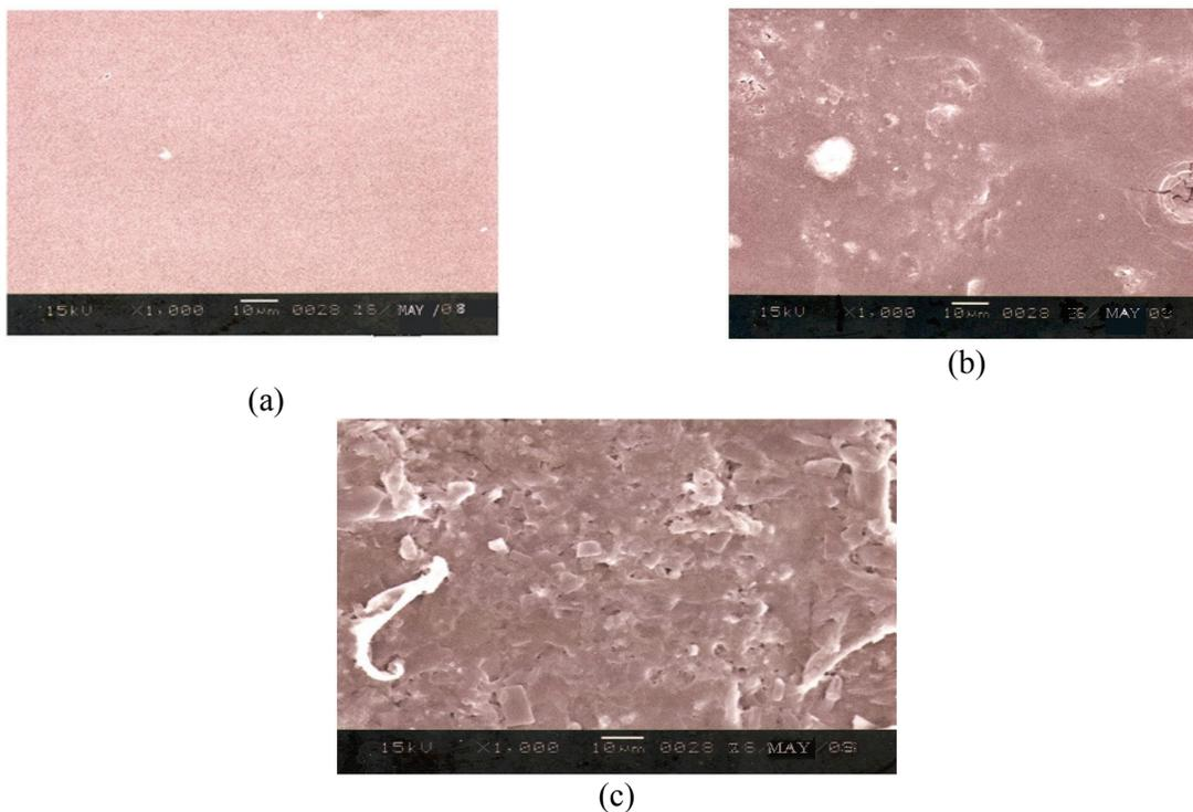
Fig. 2: SEM photograph of (a) blank film; (b) carvedilol loaded film before permeation; (c) carvedilol loaded film after permeation.
