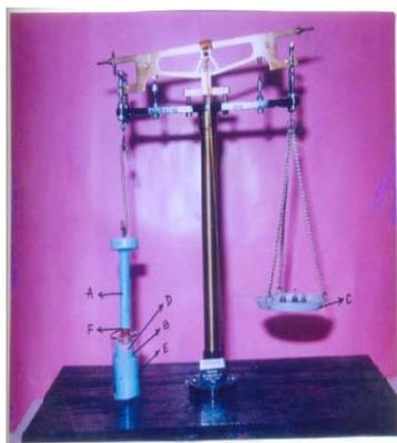
Fig. 1: Mucoadhesive test assembly
