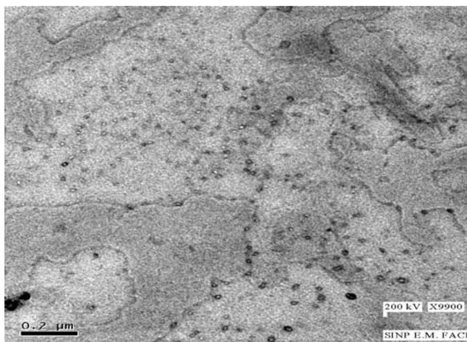
Fig. 3: Scanning electron micrograph of silver nanoparticles
