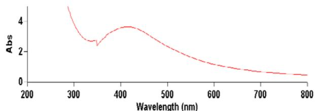
Fig. 2: UV vis absorption spectra of silver nanoparticles
