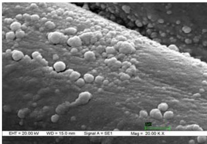
Fig. 4: Scanning electron micrograph of cotton fabric coated with silver nanoparticles
