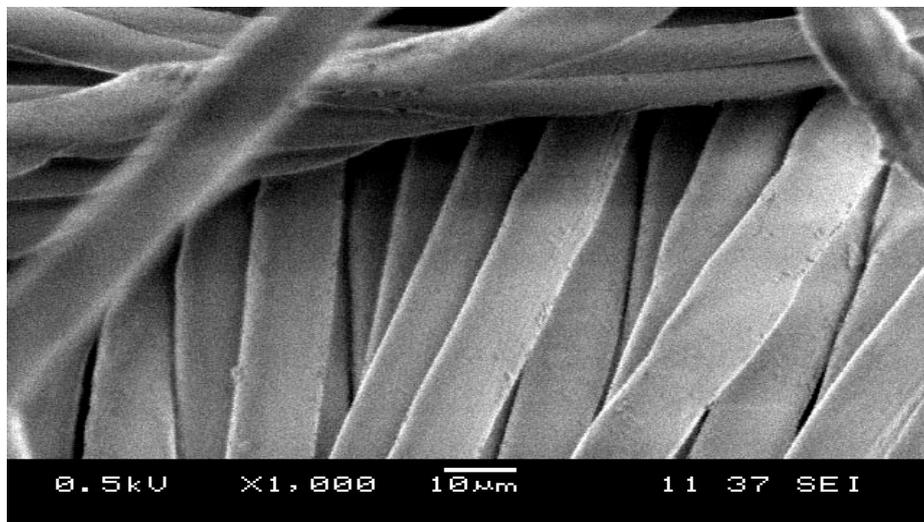
Fig. 8: SEM image of the treated 45/55% Polyester/Cotton woven
