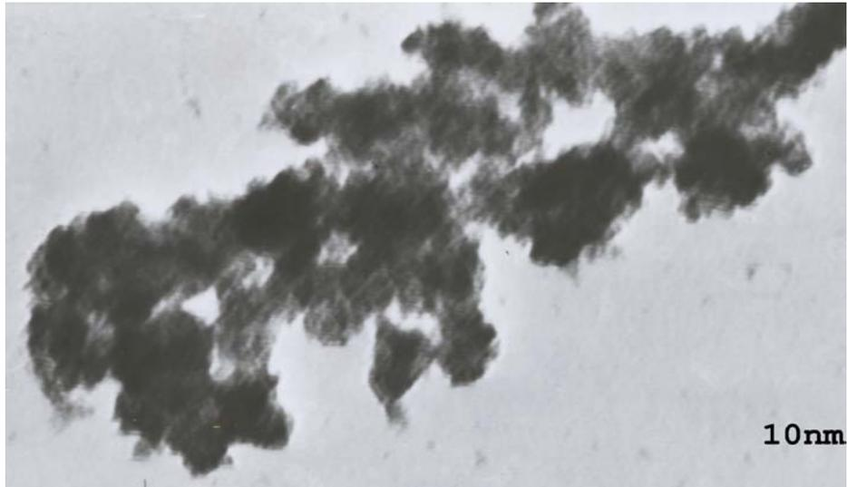
Fig. 6: TEM of Zinc oxide nanoparticle (1, 2 Ethanediol Medium)
