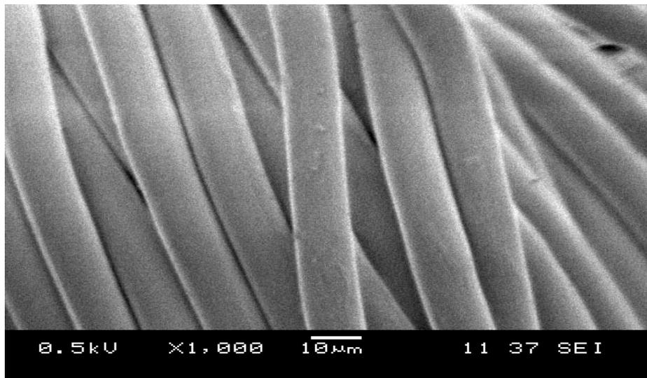
Fig. 7: SEM image of the Untreated 45/55% Polyester/Cotton woven
