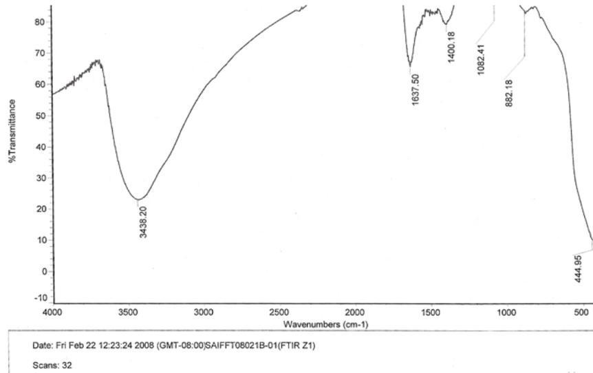
Fig. 3: FTIR of Zinc oxide nano particle (Water medium)
