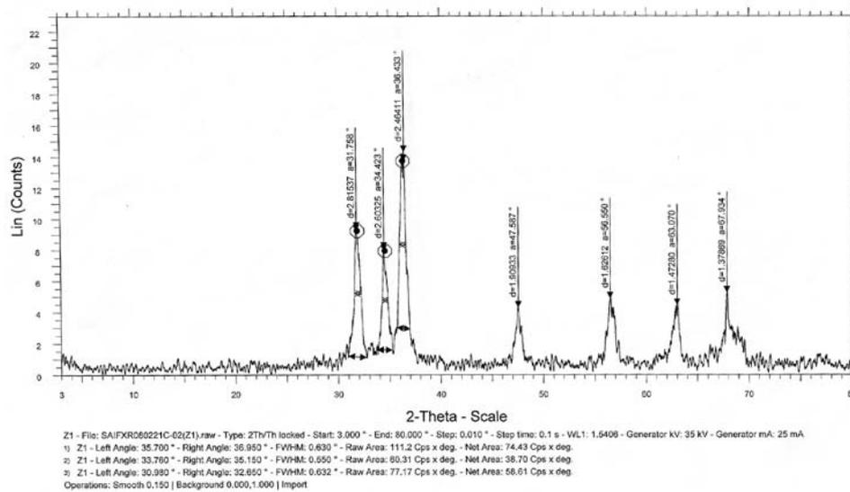
**Fig. 1: XRD of Zinc oxide nano particle (Water medium)**
