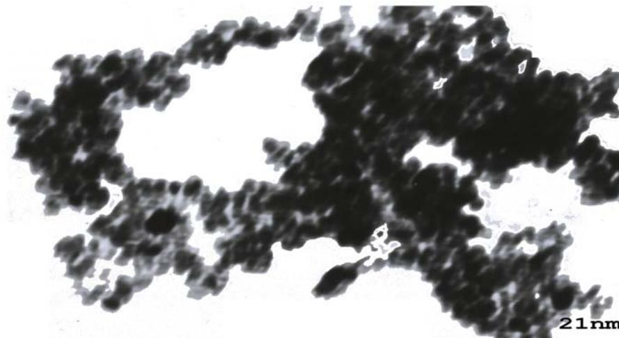
Fig. 5: TEM of Zinc oxide nanoparticle (water Medium)
