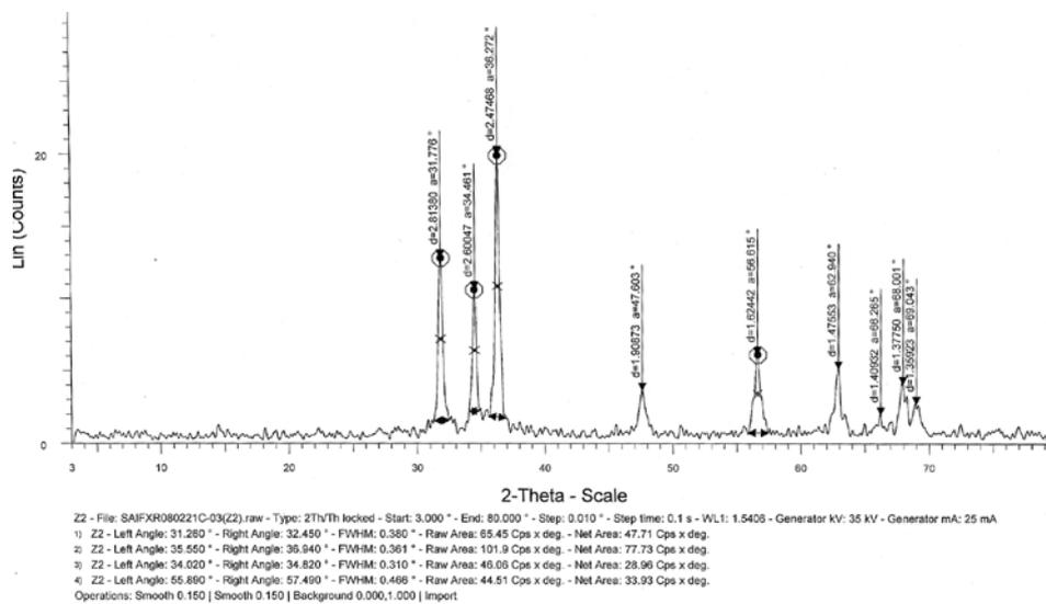
**Fig. 2: XRD of Zinc oxide nanoparticle (1, 2 Ethanediol medium)**
