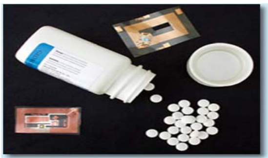
Fig. 6: RFID placed behind label on pharmaceutical 19
