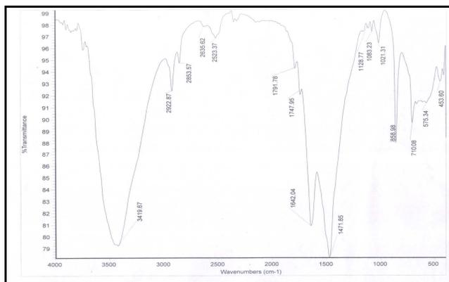
Fig. 2: FT-IR spectrum of chitin from *D. scortum* shell
