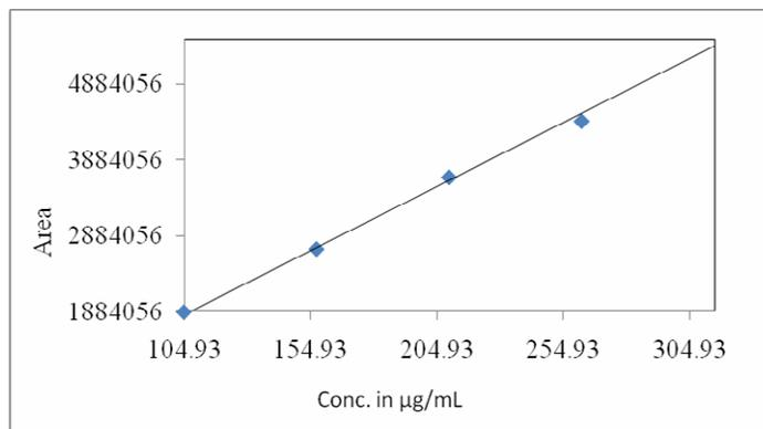
Fig. 3: Calibration curve for ZHM
