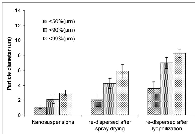
Fig. 3: LD particle sizes of ibuprofen nanosuspension and re-dispersed ibuprofen after spray drying and lyophilization
