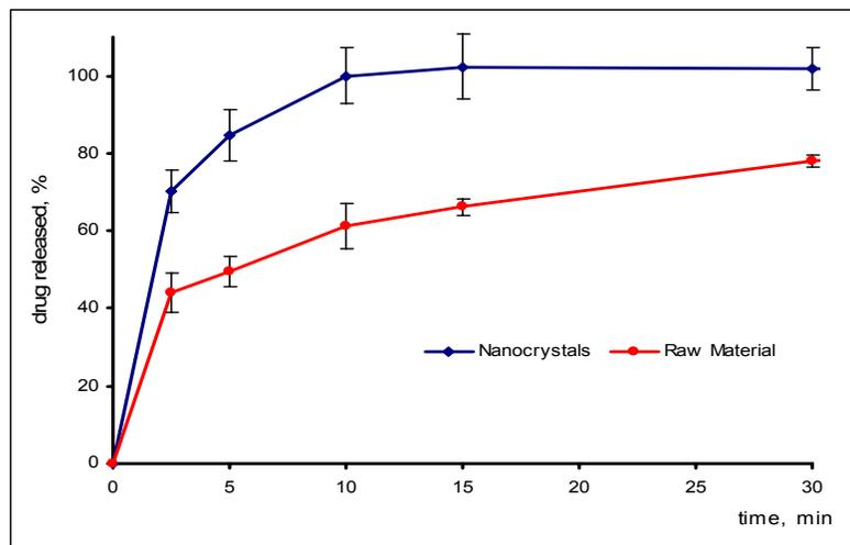
**Fig. 6:** Dissolution velocity profile of raw material (mean size d50%: 56 µm, LD) and ibuprofen nanocrystals (mean size: 929 nm, PCS) in water
