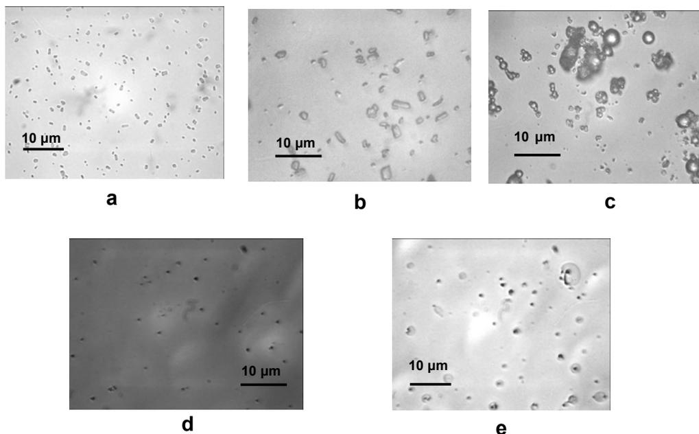
Fig. 7: Light microscopic pictures of ibuprofen nanosuspension (a), dried nanocrystals after spray-drying (b), dried nanocrystals after lyophilization (c), re-dispersed nanocrystals from pellets (d) and re-dispersed nanocrystals from effervescent granule (e)
