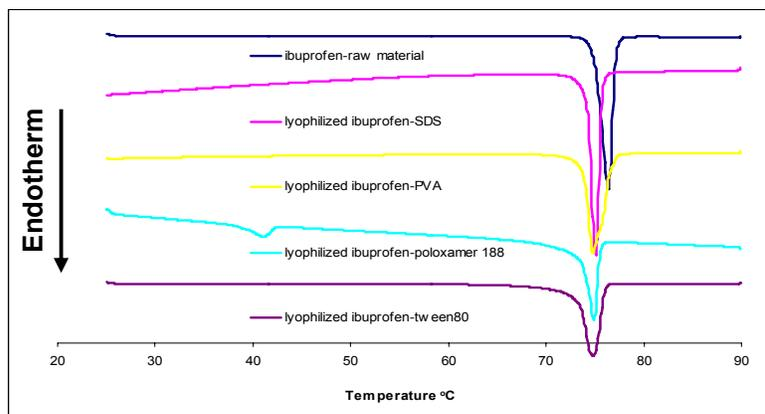
Fig. 4: Influence of stabilizers on fusion temperature and crystallinity of lyophilized ibuprofen nanocrystals
