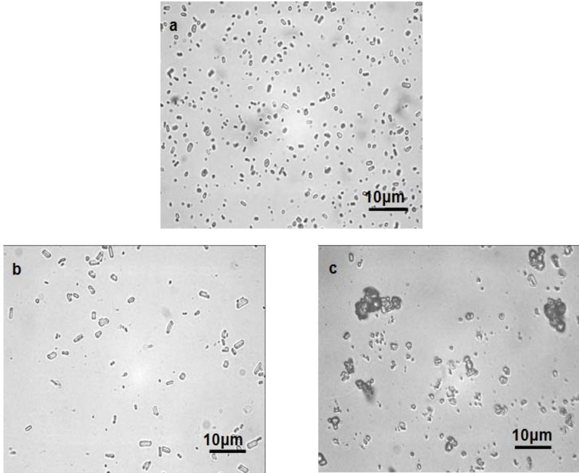
Fig. 2: Light microscopic pictures of ibuprofen nanosuspension after production (a), re-dispersed ibuprofen nanocrystals after lyophilization (b) and re-dispersed ibuprofen nanocrystals after spray drying (c)
