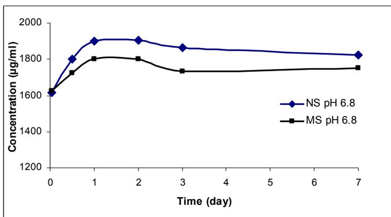
Fig. 5: Saturation solubility of ibuprofen nanocrystals and raw materials in buffer having a pH of 6.8 at 25°C
