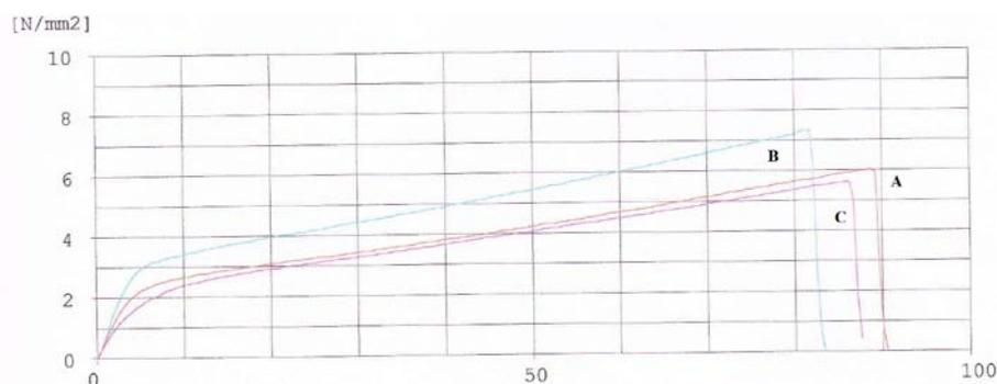
**Fig. 6:** Strain stress relationship of films of formulations of (A) Film containing only polymer (P2) (B) Film containing polymer, plasticizer and modifiers (P11) (C) Film containing polymer, drug and other excipients (P16).
