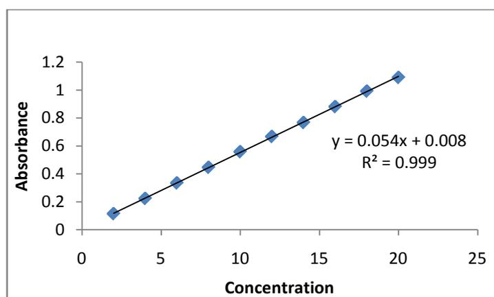
**Fig. 3: Calibration curve of Quercetin on U.V. spectrophotometer.**
