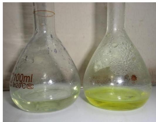
Fig. 2: It Shows the Test for Free Formaldehyde of Prepared Implants (70:30)
