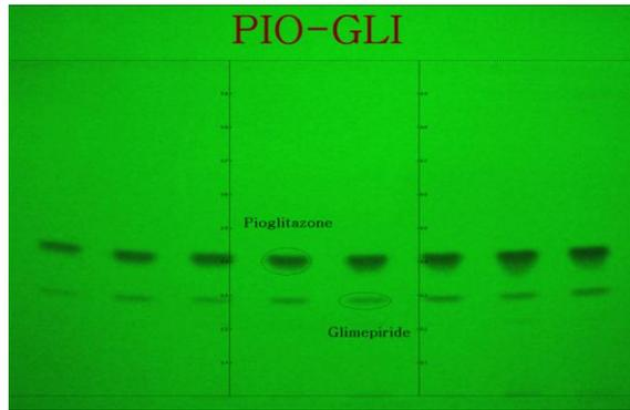
Fig. 1: HPTLC plate with eight tracks of mixture compound
