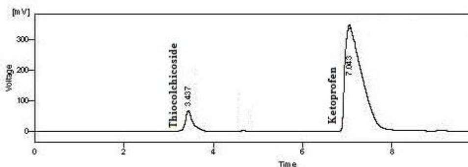
**Fig. 2: Chromatogram of Thicolchicoside and Ketoprofen. Mobile phase :Ammonium acetate buffer:acetonitrile:methanol(50:30:20,v/v).Flow rate:1.2 ml/min,injection volume:20µl column:C18 (Enable C18 G)(250 mm x 4.6mm,5µ).UV detection 310**
