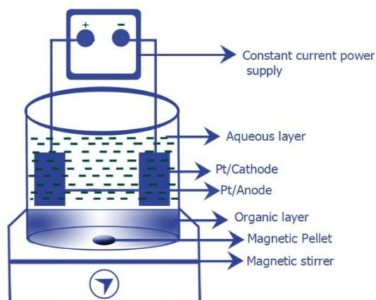
**Fig. 1: Experimental Cell set up for the oxidation 4-methylbenzyl alcohol by Biphasic electrolysis.**
