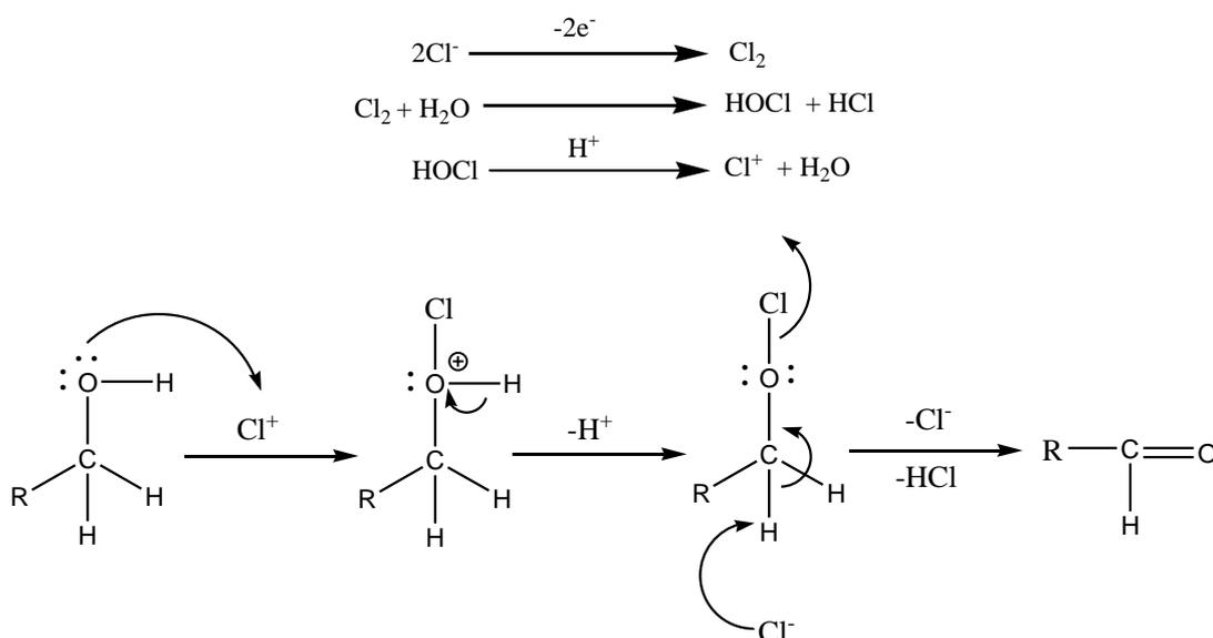
Scheme 2: The Possible mechanism for the biphasic electrolysis of 4-methylbenzylalcohol.
