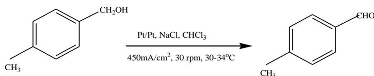
Scheme 1: Electrochemical oxidation of 4-methylbenzylalcohol by biphasic electrolysis.
