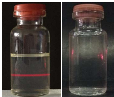
Fig. 1: The appearance of nanoemulsion containing solid dispersion of BSA and artin-M (left) and water (right). Each container was irradiated by red laser light. The red light path was only observed within nanoemulsion media due to the reflection of light by the Tyndall effect of the globules.
